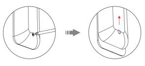
1. Loosen the screw on the back of the remote with a screwdriver.
